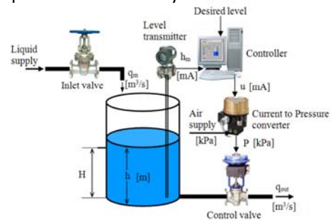
Figure 1 Automatic level control system
